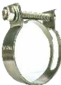
*Aço zincado**Torque de aperto: 100 kg/cm**Largura fita: 20 mm*
